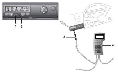
To connect the diagnostic device to the DTCO 1381:
